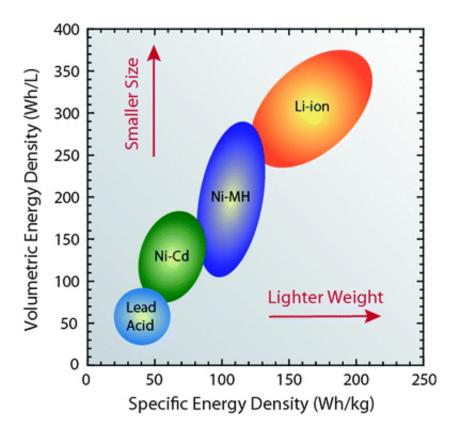
Now, once capacity is assessed, empirical values for specific mass  $(m_{spec})$  (measured in *Wh/kg*) are used to estimate the mass with the following formula:
